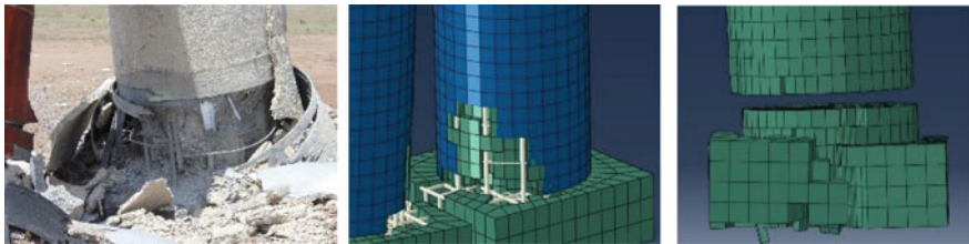
Fig. 7 Visual comparison of actual test (left) and simulation with (middle) and without retrofitting (right)
