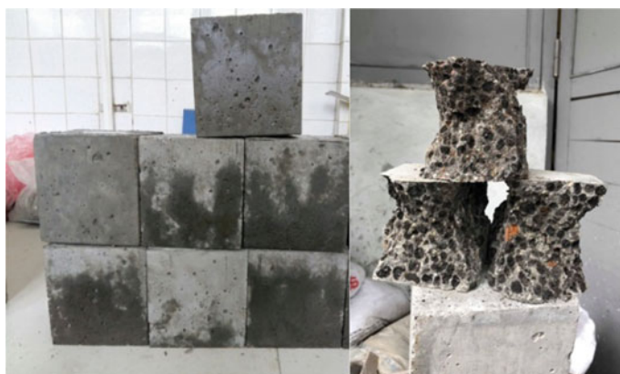
Fig. 2 Concrete samples for compression test
