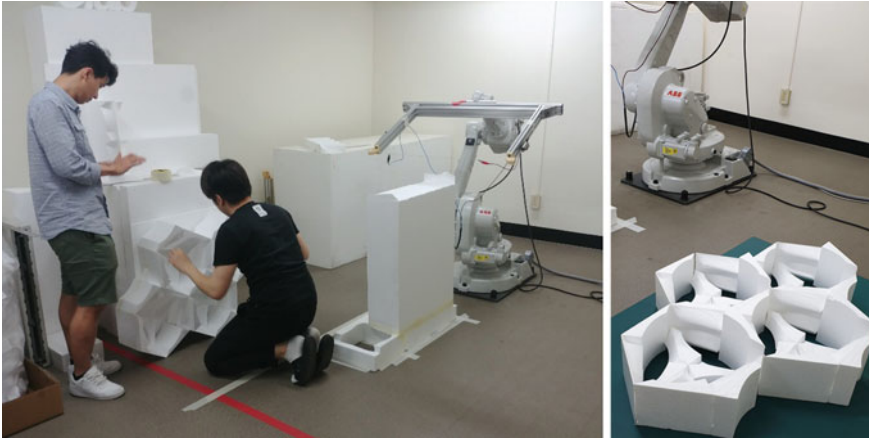
Fig. 8 Modular unit screen fabricated using a robotic arm where various subsymmetries are superimposed
