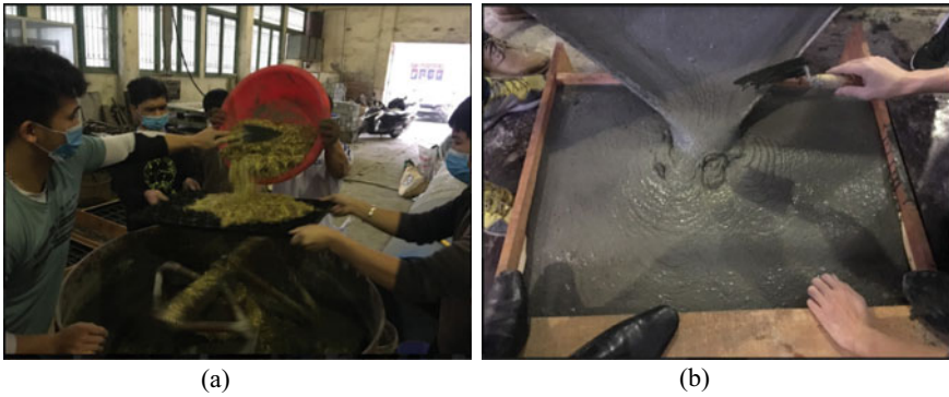
Fig. 2 a Mixing and b placing of UHPFRC mixtures
