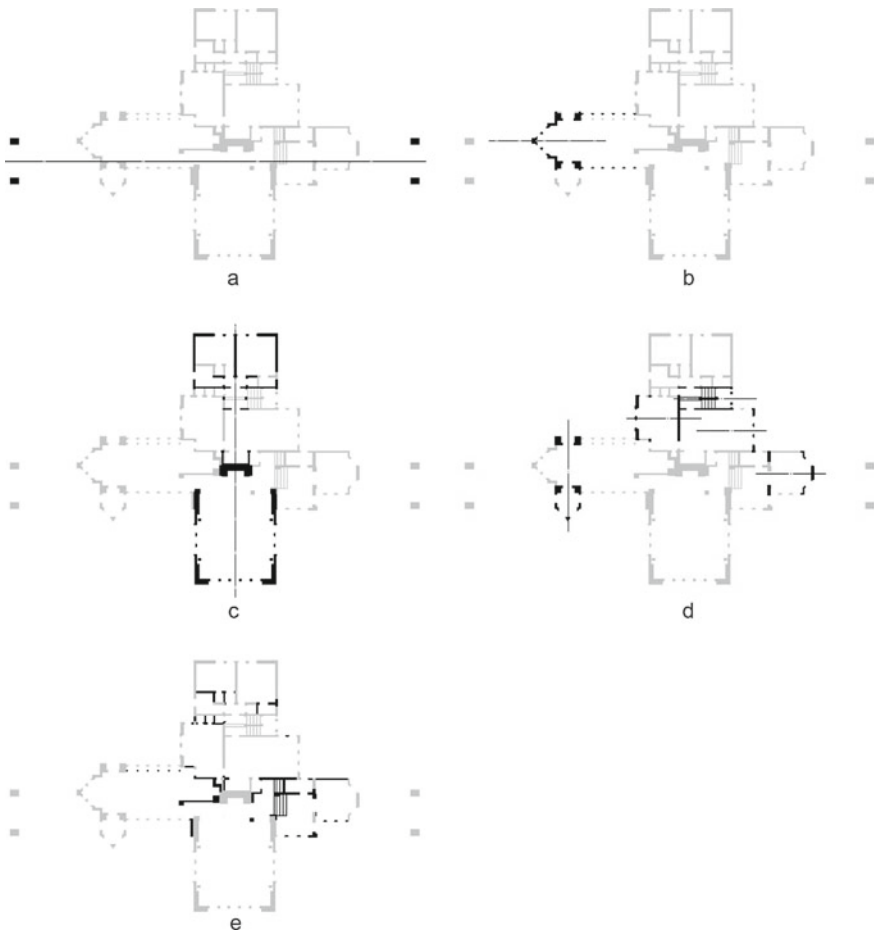
Fig. 3 Partial ordering with regard to subsymmetry drawings for the first floor plans of the Ward Willits House, 1901, Highland Park, Illinois: a long axis through porch piers; b axis through the dining room; c axis through the living room and hearth. A hearth facing into the living room is at its center; d minor axes through various parts of the plan; e remaining elements having no overall symmetry
