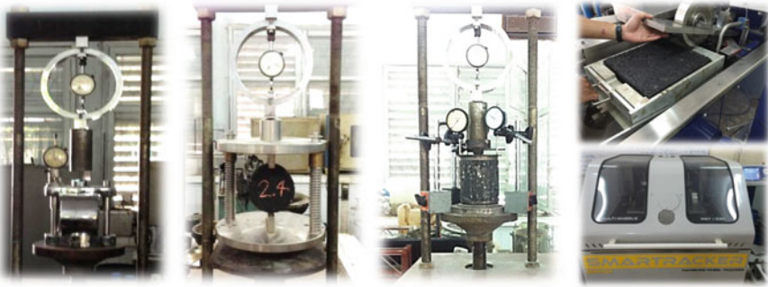
Fig. 5 Set-up for Marshall stability, indirect tensile strength, resilient modulus, and wheel tracking test (from left to right)
