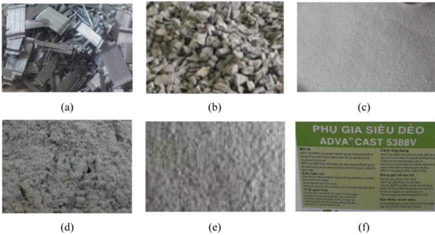
Fig. 2 SFRC materials: a Steel fibers, b Aggregate, c Fine sand from Binh-Dinh province, d Fly ash, e Silica fume, f Plasticizer
