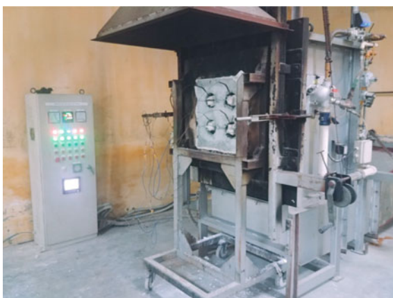
Fig. 3 Specimen is set in the burning room
