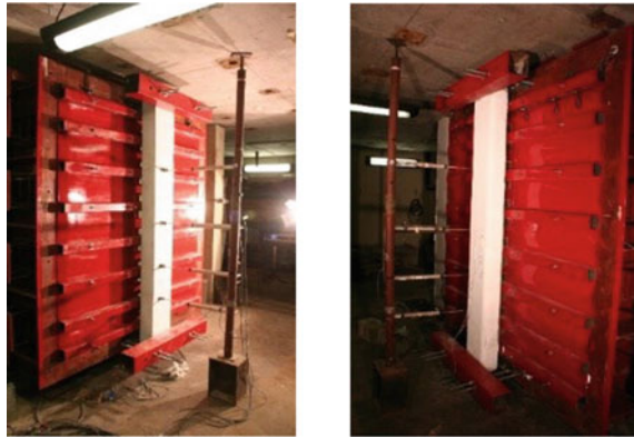
Fig. 1 Shock tube test set up for control column (left) and retrofitted column (right)
