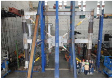
(c) Phase 2 test (2% second floor drift)
