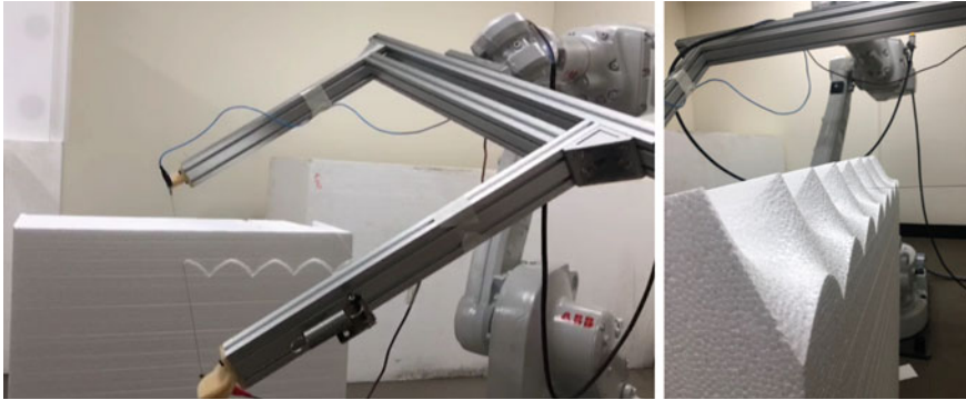
Fig. 7 Component unit cutting with the hot wire
